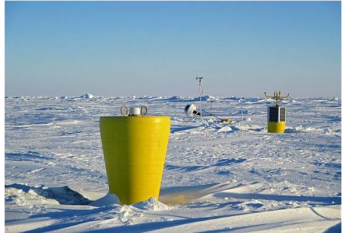
This ITP was installed in the Beaufort Sea in March 2014 to collect data on complex air-ice-ocean interactions that govern sea ice formation and retreat. Credit: John Kemp/WHOI
