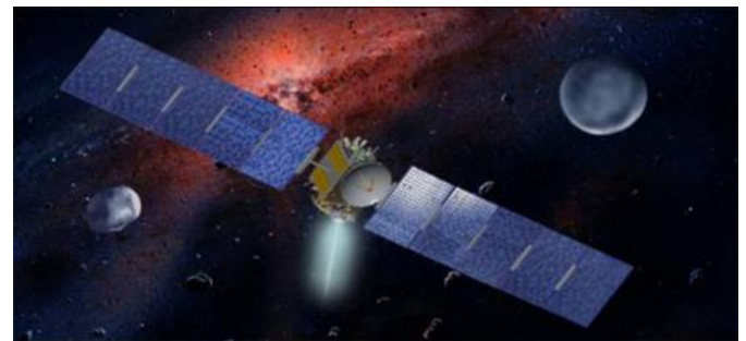
The Dawn spacecraft, equipped with large solar panels to power its electrical engine. Credit: NASA
