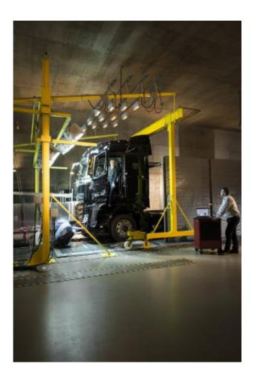
To test air conditioning systems, the driver's cab is exposed to realistic conditions. Credit: Markus Breig, KIT
