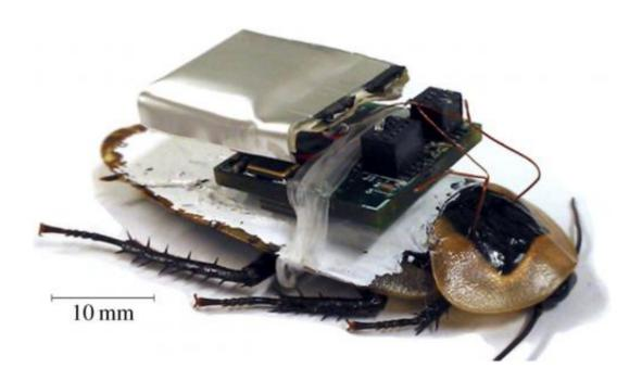
Discoid cockroach with attached electronic backpack (battery on top, board attached to the forewings). The electrodes enter the body through the pronotum. Credit: *Journal of the Royal Society Interface*, DOI: 10.1098/rsif.2014.1363
