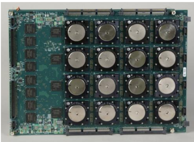
Neuromorphic chip with a maximum load—equivalent to 400 billion synaptic operations per second per watt. Credit: Day Donaldson, CC BY
