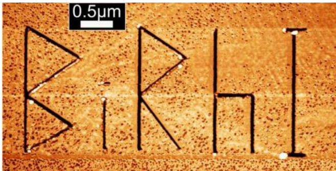
Microscopic image of the topological insulator Bismuth-Rhodium-Iodine (Bi 14 Rh 3 I 9 ). The engraved letters BiRhI act as artificially introduced steps at the crystal surface. Credit: M. Morgenstern, RWTH Aachen
