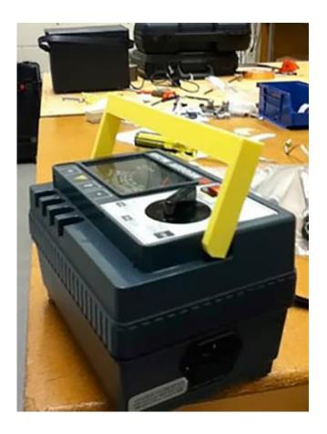
This 3-D printed part replaced the meter's original handle. Credit: Princeton Plasma Physics Laboratory
