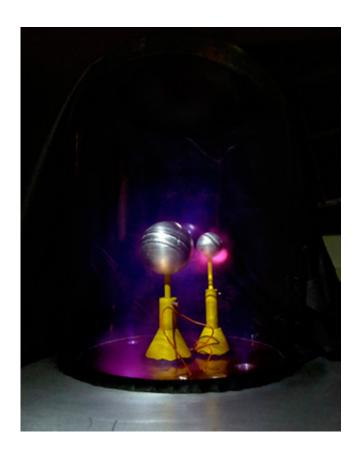
3-D printed parts provide the stands for the aluminum globes in PPPL's Planeterrella, a device that simulates Northern Lights. Credit: Princeton Plasma Physics Laboratory
