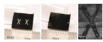
For an experiment to recover serial numbers that have been destroyed, NIST researchers hand-stamped X imprints into stainless steel (first image) to simulate a firearm serial number. Then they polished away the imprints (second image, scale bar in millimeters). Researchers recovered the imprints (third image) by combining pattern quality maps, calculated by software, which reveal crystal damage and deformation in the steel.
