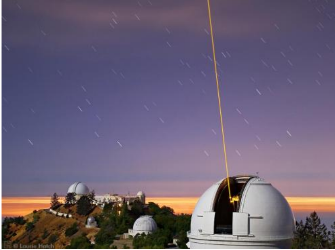
Telescope using laser guide star adaptive optics at UC's Lick Observatory. Credit: Laurie Hatch photo
