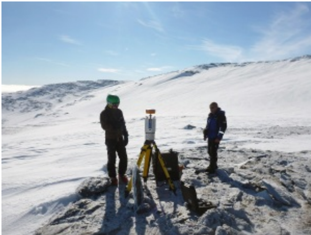
Laser scanning the Kringsollfonna ice patch to measure how much snow accumulates in the winter and melts in the summer. Credit: Geir Vatne, NTNU
