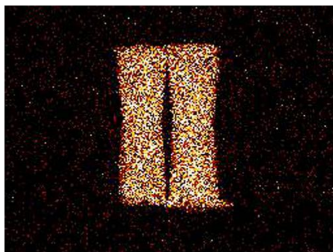
Energy-dispersive X-ray spectroscopy data of elemental zinc in the micromotors. Credit: Jacobs School of
