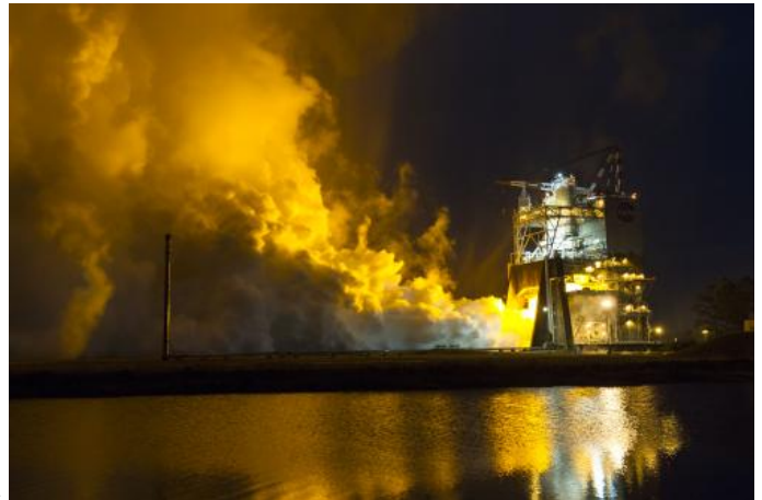
The RS-25 engine fires up for a 500-second test Jan. 9, 2015 at NASA's Stennis Space Center near Bay St. Louis, Mississippi. Credit: NASA
