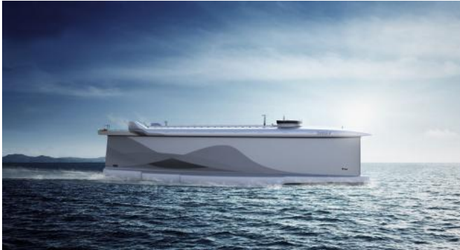
The hull of the cargo ship Vindskip TM acts as a large wing sail. Credit: LADE AS
