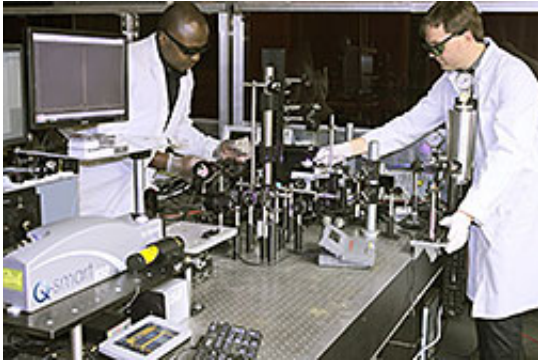
NETL researchers Christian Goueguel (left) and Cantwell Carson align and operate NETL's laser induced breakdown spectroscopy (LIBS) equipment in a lab experiment.
