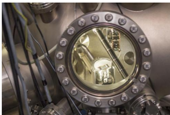
Iron oxide sample in the vacuum chamber. Credit: TU Wien
