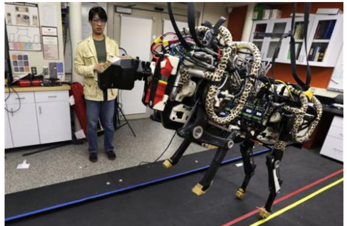
In this Sept. 30, 2014 photo, professor Sangbae Kim controls a robotic cheetah on a treadmill at the Massachusetts Institute of Technology in Cambridge, Mass. MIT scientists said the robot, modeled after the fastest land animal, may have real-world applications, including for prosthetic legs. (AP Photo/Charles Krupa)
