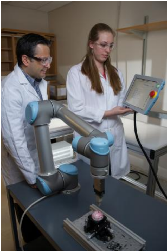
Facundo Fernandez (left) and Rachel Bennett, use a robotic arm to probe objects with irregularly-shaped surfaces for mass spectrometry. Credit: GA Tech
