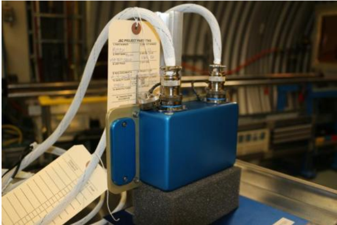
The Battery-operated Independent Radiation Detector (BIRD) flight unit. Credit: Courtesy of NASA
