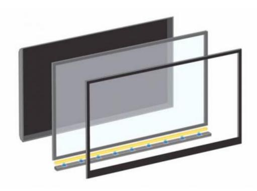
Manufacturers implement the Color IQ component (shown here as a thin, yellow bar) into their televisions during the normal construction process, but use blue LEDs (blue dots) in place of the standard white LED back lights. Credit: QD Vision
