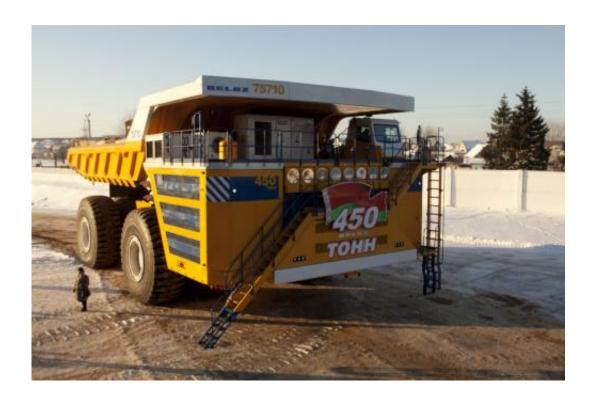
The world's biggest truck has an electric drive system. Four electric machines with 1,200 kilowatts each from Siemens help the 800 ton gigant moving. Recently, the first truck of the BelAZ 75710 series went into operation in a sibirian mine in the Kuzbass region. The truck is more than 20 meters long, 10 meters wide and has a height of 8 meters. It weighs 360 tons without load and can transport 450 tons of material. This amount is equal to the weight of a fully loaded Airbus A380.
