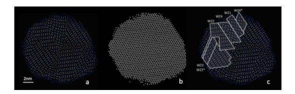
These are three atomic-resolution views of a copper-indium-sulfur nanoparticle: (a) Only the copper and indium atoms are shown in blue and yellow; (b) Copper and indium atoms are shown in same color demonstrating that they form a perfect hexagonal lattice; (c) Same as (a) with the boundaries between regions of distinct copper-indium order outlined. Credit: Xiao Shen, Vanderbilt University
