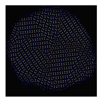
A Scanning Transmission Electron Microscope image of a copper-indiumsulfide nanoparticle that shows the interlaced crystalline structure. Credit: Wu Zhou, Oak Ridge National Laboratory
