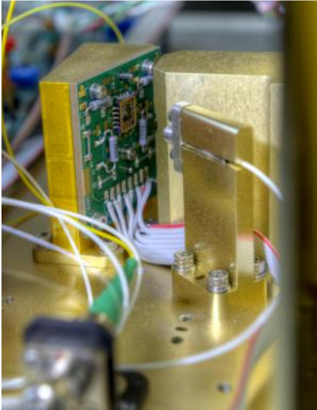
The micro-electro-mechanical — or MEMS — mirror at the center of the circuit board provides the scanning function in the Goddard Rendezvous Solid-state Scanning Lidar. Credit: NASA/W. Hrybyk
