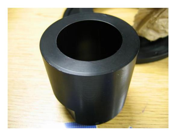
This is a close-up view of a baffle that will be coated with a carbon-nanotube coating. Credit: NASA Goddard/Paul Nikulla
