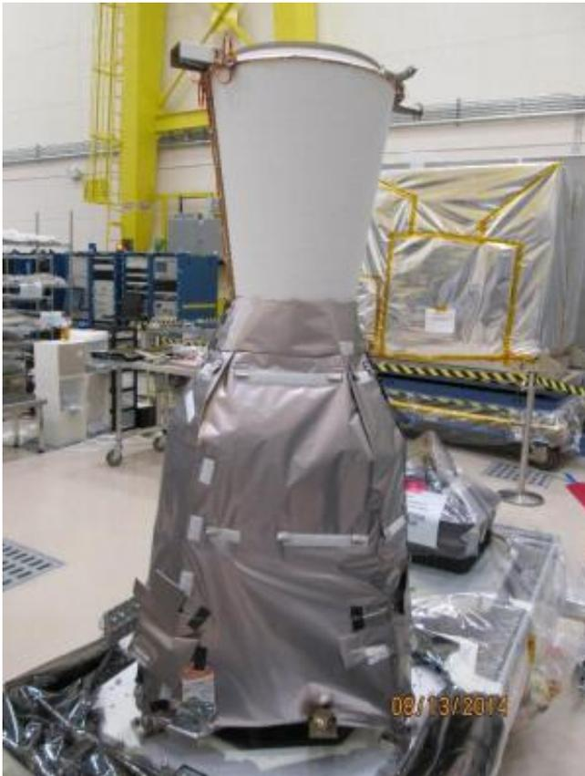
The GOES-R GLM Sensor Unit with thermal blankets and (non-flight) baffle installed. This is what the GLM Sensor Unit will look like when it is on the spacecraft. Credit: Lockheed Martin
