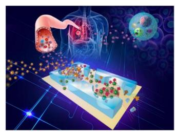
The prototype lab-on-a-chip is made of a widely used silicone rubber called polydimethylsiloxane and uses a technique called 'on-chip immunoisolation.' Credit: University of Kansas/KU News Service
