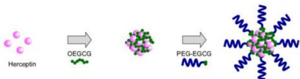
Image 1: A schematic diagram of the two-step assembly process of the core-shell structure of the green tea drug carrier. The core of this carrier is made of OEGCG and Herceptin, a protein drug currently used to treat breast cancer. Surrounding the EGCG-Herceptin core is a shell containing PEG-EGCG.
