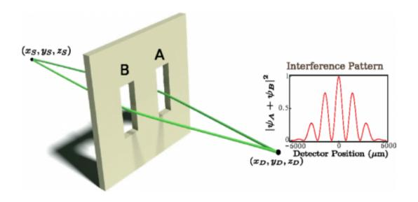
Two-slit experiment. Inset shows a typical interference pattern obtained by assuming  $\psi AB = \psi A + \psi B$ . Credit: Source: R. Sawant, J. Samuel, A. Sinha, S. Sinha, and U. Sinha, Nonclassical Paths in Quantum Interference Experiments, *Phys. Rev. Lett.* 113, 120406 (2014).
