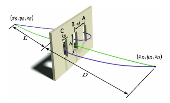
Path integrals in a lab. The green line demonstrates a representative classical path. The purple line demonstrates a representative nonclassical path. The various length parameters are marked; d designates the interslit distance, w designates the slit width, h designates the slit height, L designates the distance from the source to the slit plane, and D designates the distance from the slit
