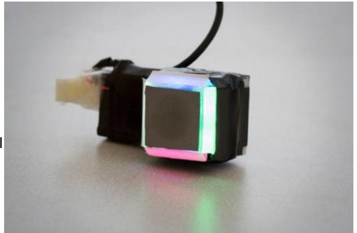
The GelSight sensor uses different-colored light, channeled down different faces of the cubic housing, to make three-dimensional measurements. Credit: Melanie Gonick/MIT
