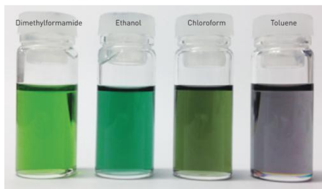
Figure 1: Different solvents can cause benziphthalocyanine to shift between its strongly aromatic quinoidal form and its weakly aromatic phenol form, which changes the color of the solution. Credit: Atsuya Muranaka, RIKEN Center for Sustainable Resource Science
