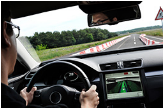
PRORETA in use: The driving corridor is displayed while driving through road works. Picture: Continental.
