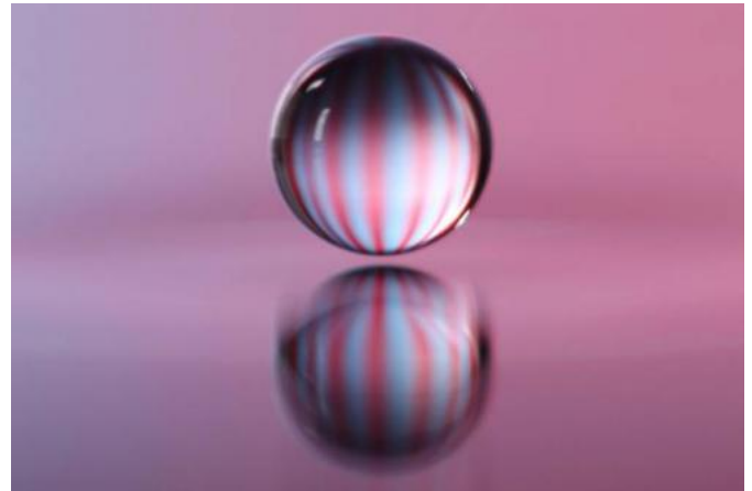
Close-ups of an experiment conducted by John Bush and his student Daniel Harris, in which a bouncing droplet of fluid was propelled across a fluid bath by waves it generated. Credit: Dan Harris
