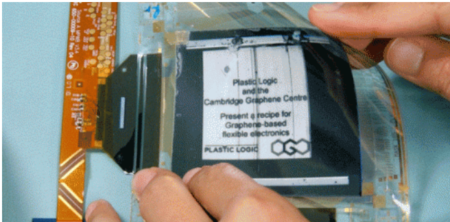
Active matrix electrophoretic display incorporating graphene. Credit: Plastic Logic
