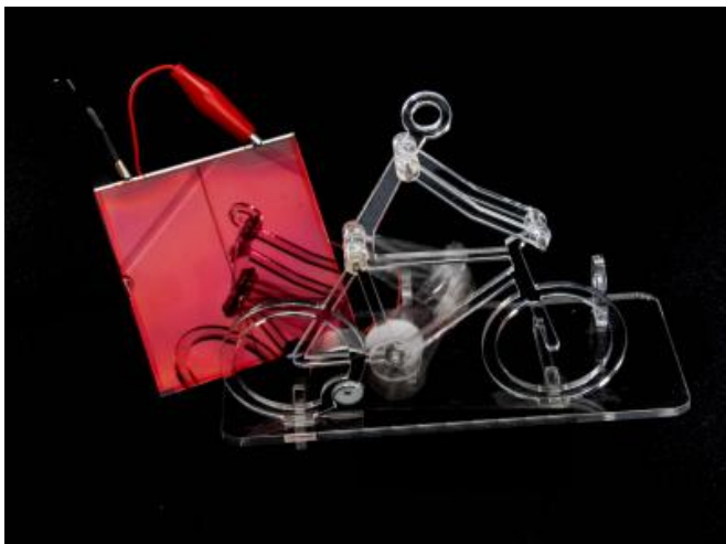
A module to which two cells have been connected in series, powering a toy. Credit: IK4-Ikerlan
