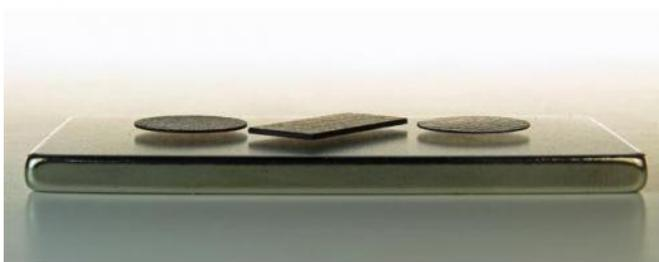
Three pieces of pyrolytic graphite are levitated freely over a single multipole NdFeB magnet
