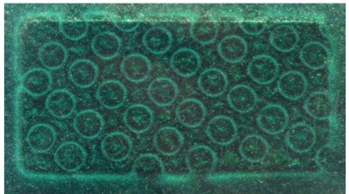
Magnetic field domain pattern of a printed multiple NdFeB magnet, revealed by magnetic field viewing film
