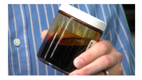
Derived from plants, bio-oil can be processed into gasoline, diesel or other typical petroleum products such as plastics. Credit: PNNL/Eric Francavilla
