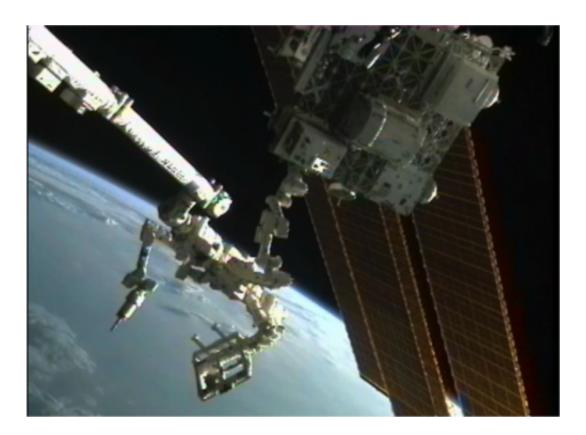
A new complement of hardware will outfit NASA's Robotic Refueling Mission (center on International Space Station platform) for a fresh set of satellite-servicing demonstrations. Credit: NASA
