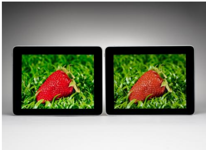
Quantum dots make greens and reds pop on screens (left) compared with other types of displays (right). Credit: Credit: 3M
