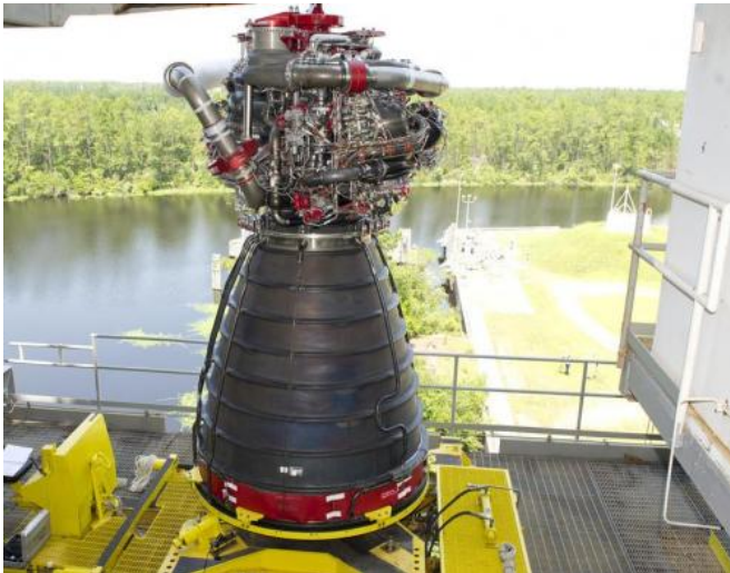
RS-25 rocket engine No. 0525 is positioned onto the A-1 Test Stand at NASA's Stennis Space Center in Mississippi in preparation for a series of developmental tests. Credit: NASA
