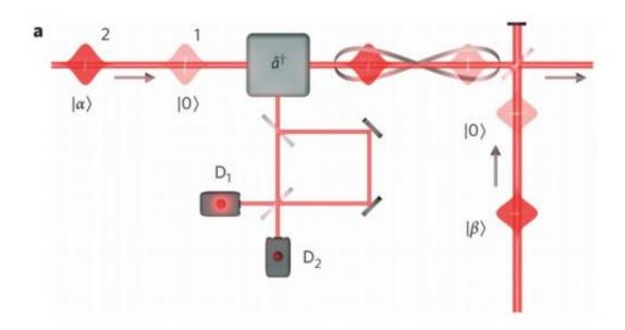
Illustration of the proposed scheme to generate hybrid entanglement of light (a single photon and a coherent wave-like state of light). Credit: Jeong, et al. ©2014 Nature Photonics
