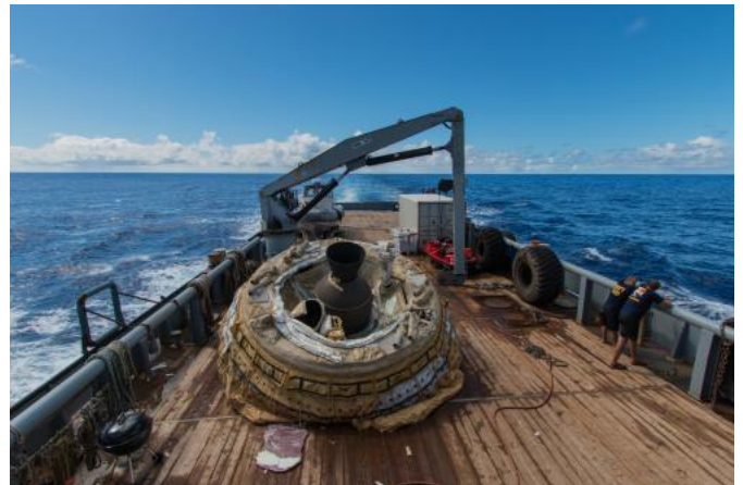
The first "flown" test vehicle of Low-Density Supersonic Decelerator project relaxes aboard the recovery vessel Kahana. During the June 28, 2014, engineering flight, the saucer-shaped test vehicle climbed to over 180,000 feet (about 55,000 meters) in altitude and went as fast as four times the speed of sound. Credit: NASA/JPL-Caltech
