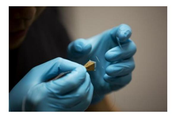
Jaesang Lee, Electrical Engineering PhD Student and member of the Stephen Forrest's Optoelectronic Components and Materials Laboratory, constructs a light concentrating LED in the EECS Building on May 29, 2014. The LED is able to both generate and emit light through its pyramidal shape, enabling for efficient energy use. Credit: Joseph Xu, Michigan Engineering Communications & Marketing
