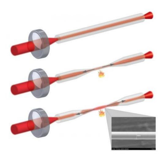
This image depicts light propagating through an optical nanofiber during the pulling process with a SEM image of the 536 nanometer diameter waist. Credit: J. E. Hoffman and E. Edwards, JQI at UMD
