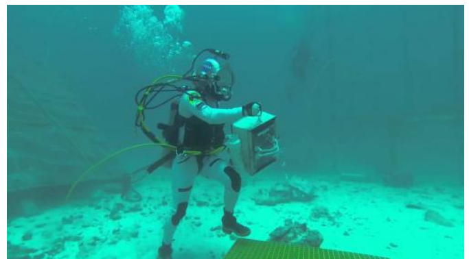
A simulated spacewalk during NASA's Seatest to practise moving across different terrains and deploying sensor arrays. At different points, the astronauts ran through ways of sampling the seabed. Techniques included a simple inverted bag, a modified 'pooper-scooper' and an advanced pneumatic drill that chips away at a rock while ensuring that pieces do not fly away. Credit: ESA
