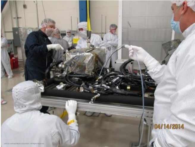
This image shows the EXIS instrument being installed onto the sun pointing platform of the GOES-R spacecraft. Credit: Lockheed Martin
