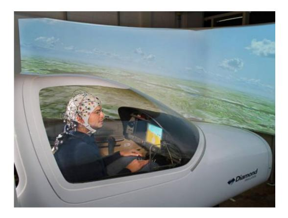
Simulating brain controlled flying at the Institute for Flight System Dynamics. Credit: A. Heddergott/TU München
