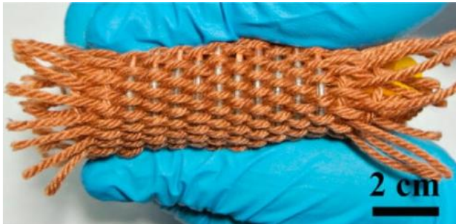
Fiber-shaped full lithium-ion batteries that are woven into a textile hold promise for powering wearable electronics. Credit: Weng, et al. ©2014 American Chemical Society
