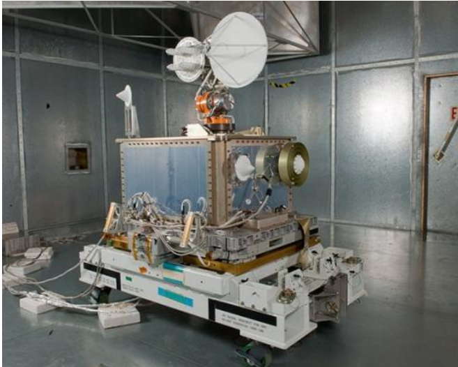
The SCaN Testbed, operating aboard the International Space Station, features two S-band and one Ka-band software defined radios, which will help NASA demonstrate advanced communications, networking and navigation tools in space. Credit: NASA
