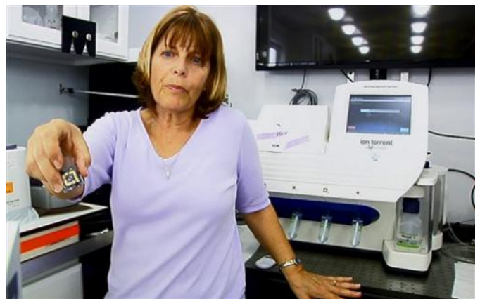
This image from video, taken March 29, 2014, shows University of Florida molecular biologist Andrea Kohn in front of a genomic sequencing machine attached to a special tilting tabletop that bobs with rough waves in this shipboard laboratory during a sail in the Gulf Stream off the coast of Florida. The lab is part of a research project to decode the genomic blueprints of fragile marine life in real time -- on board the ship where they were caught. (AP Photo/Suzette Laboy)
