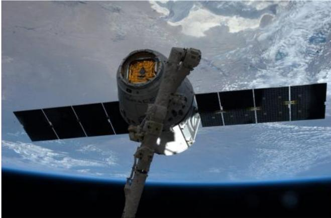
Flight Engineer Steve Swanson sent this image of the SpaceX Dragon grappled by Canadarm2, a robotic arm on the exterior of the International Space Station. Credit: NASA
