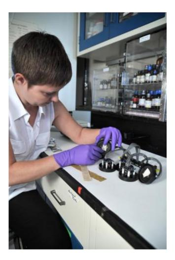
Dr. Brandy White inserts a porphyrin-functionalized, paper sensor surface into a reflectance sensor. NRL is developing sensors that "will Wi-Fi communicate so you can use them for perimeter monitoring." Credit: U.S. Naval Research Laboratory/Jamie Hartman
