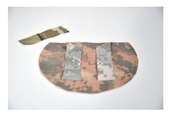
Dr. Brandy White's sorbent-porphyrin materials work for fabrics, and can be coated on hard surfaces or used in sensors. Wet or dry, "I know that you can stick them out in a July sun at 100 degrees for a week and nothing about their performance characteristics changes." She's looking into potential for biodiesel purification. Credit: U.S. Naval Research Laboratory/Jamie Hartman
